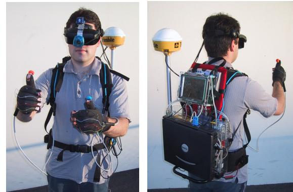
Figure 1 - Tinmth backpack with the RC200 and video overlay devices mounted at the top, and the user wearing gloves with coloured markers attached for the hardware vision tracker
