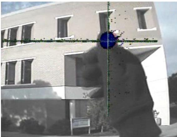
**Figure 3 - Debugging output from the RC200 showing image thresholding and the calculated marker centre point, combined with the camera view of the outdoor environment**
