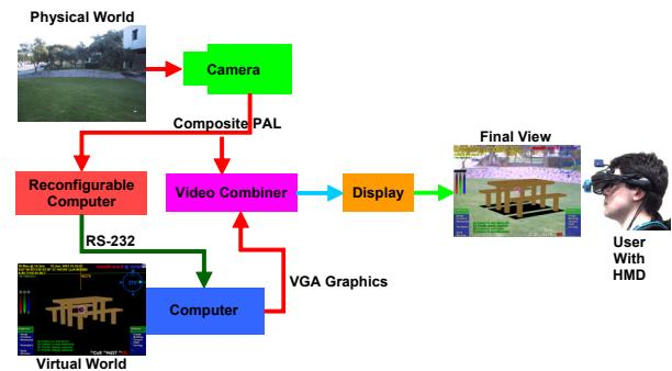
Figure 2 - Overall system schematic, showing the RC200 integrated with the general purpose laptop, and video AR implemented using hardware overlay of the two video signals
